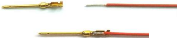
Figure 5.7 Making a communication cable
